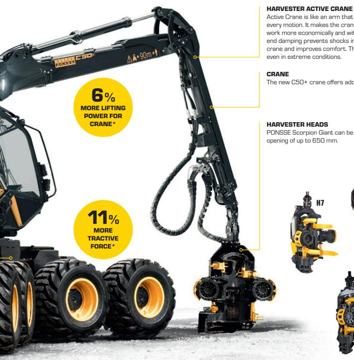
Active Crane is like an arm that can reach for the trunk without having to think through every motion. It makes the crane easier to use, helping new operators in particular to work more economically and without stressing the machine's structures. The boom's end damping prevents shocks in extreme positions. This reduces the stress on the crane and improves comfort. The solution is technically simple and remains reliable
