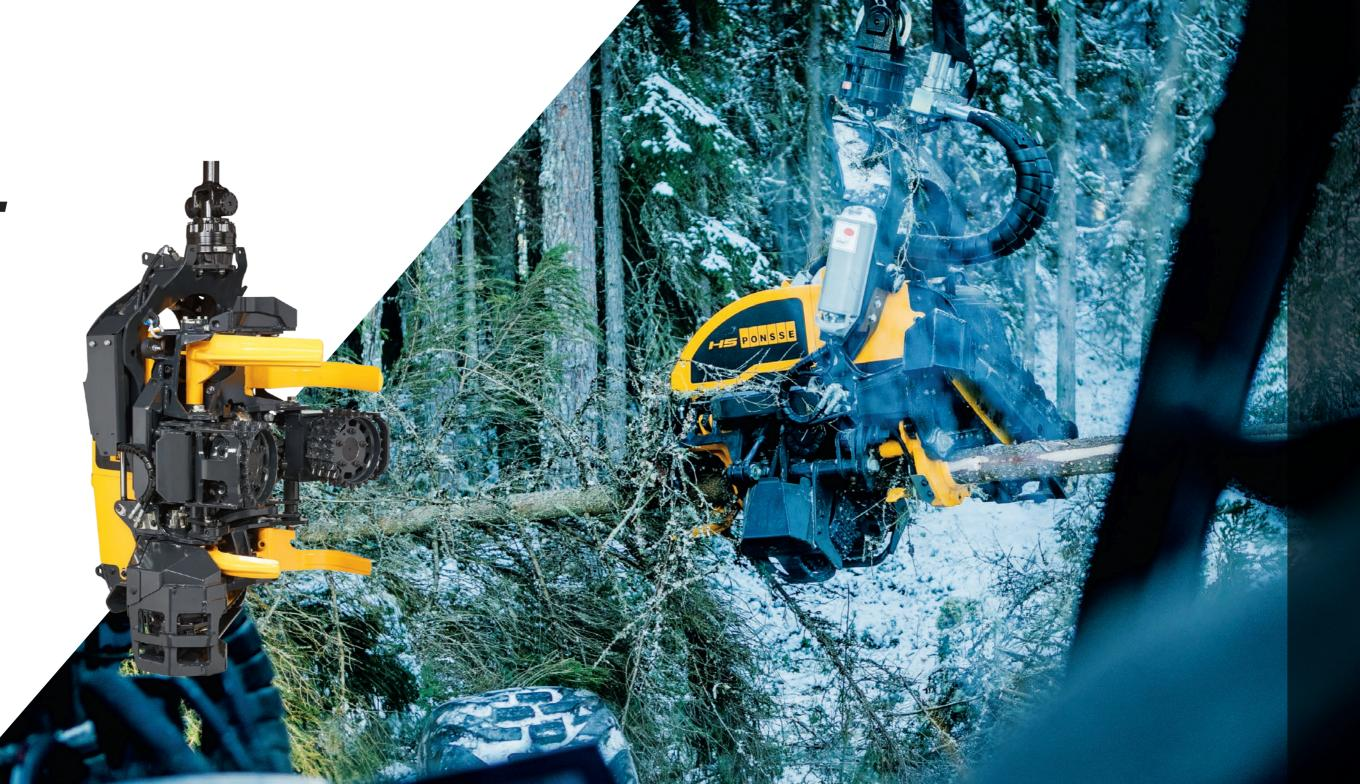
PONSSE H5 is an all-round harvester head designed specifically for efficient thinning. Its large opening range, long delimbing knives and the wide and correctly positioned upper feed roller make working at thinning sites power efficient. It is ideal when removing individual trees or collecting stems and in multi-stemming. The extremely fast yet economical feeding and sawing guarantee high productivity in all conditions.
